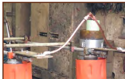
Current Cycle Test per IEEE 837-2014
