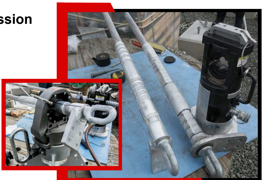
LEFT: DMC Power DC99 Full Tension dead-end with DP85 Power Unit RIGHT: Standard Crimp Compression dead-end with 60 Ton Press
