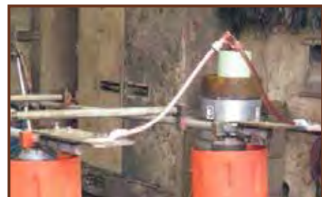
Current Cycle Test per IEEE 837-2014
