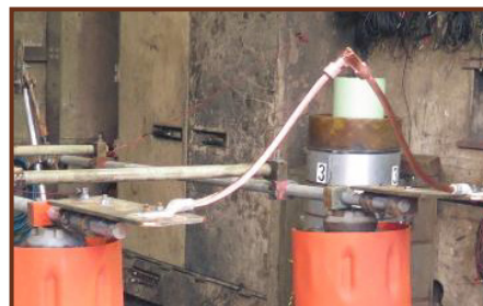
Current Cycle Test per IEEE 837-2014
