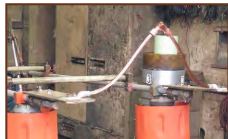
Current Cycle Test per IEEE 837-2014
