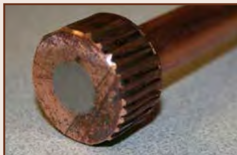
360° compression reduces voids, allowing the fitting to run cooler
