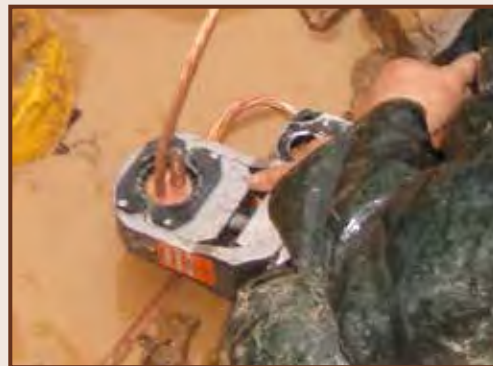
Handheld Swage Tools are compact, repeatable and easy to use in all conditions
