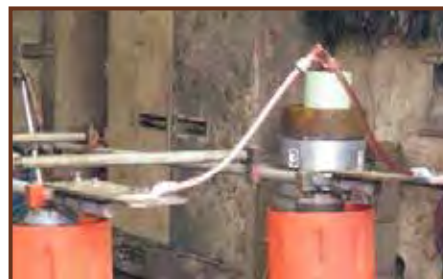
Current Cycle Test per IEEE 837-2014
